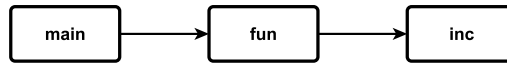
Fig. 1: The component graph corresponding to the analysis of the program in Listing 1: inc is called from fun , which is called from the program’s entry point.
